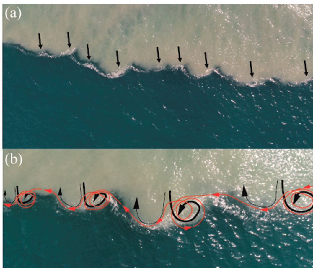
Figure 14. (a) aerial image of the undulate border of the Kodor plume on 1 September 2018 and (b) the scheme of the reconstructed circulation within the lobes (black lines) and the transport of foam and floating litter along the plume border (red lines) (b). Black arrows in panel (a) indicate foam accumulated within cyclonic vortices in the right parts of the lobes.
