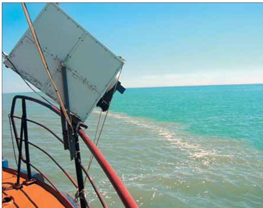
Ultraviolet fluorescent lidar measures pollution in the sea water area of the city of Sochi.
