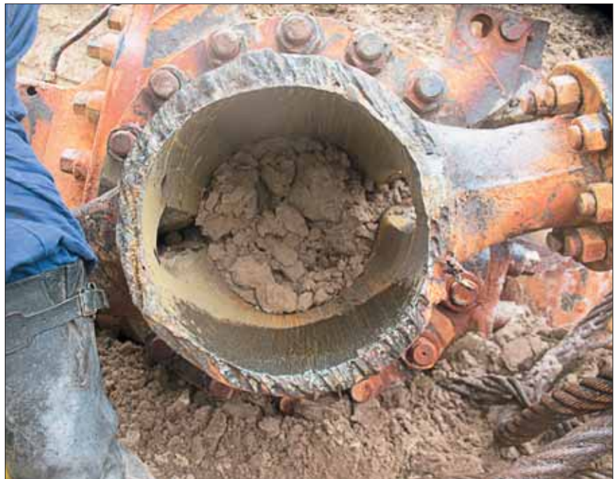
The wall thickness of a gas fitting cut off by laser of MLTK-20 varies from 30 to 40 mm.
