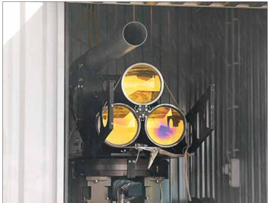
The fourth container includes a three-channel telescope with systems of a laser beam guidance to the target and of complex control, and also an operator's workstation.
