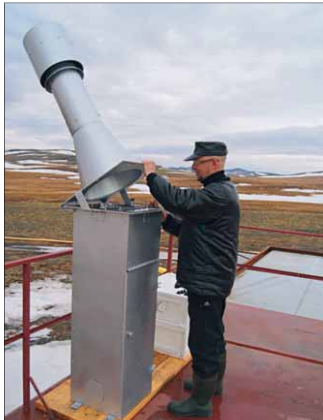
Atmospheric air sampling on the POP content at the Tiksi hydrometeoobservatory in 2010-2011.
