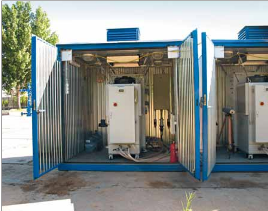
Three containers of the technological complex MLTK-20 include sources of continuous fiber laser radiation.
