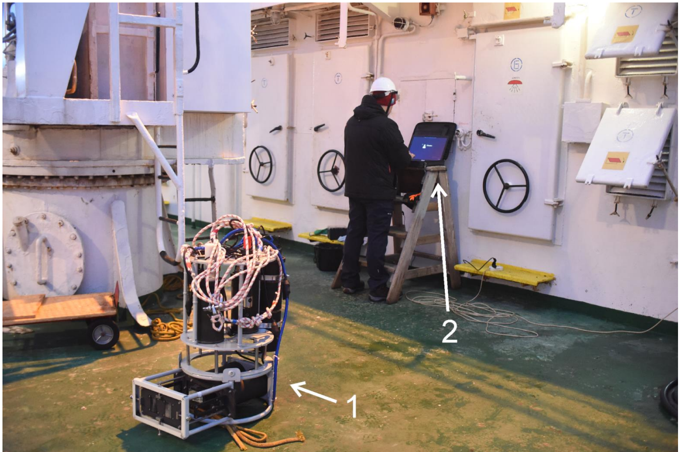
Figure 4. A hydrobiological DHC probe in combination with hydrophysical sensors of temperature, conductivity, and pressure on the deck of the Akademian Mstislav Keldysh (1). Operator’s workstation for data acquisition and processing (2).
